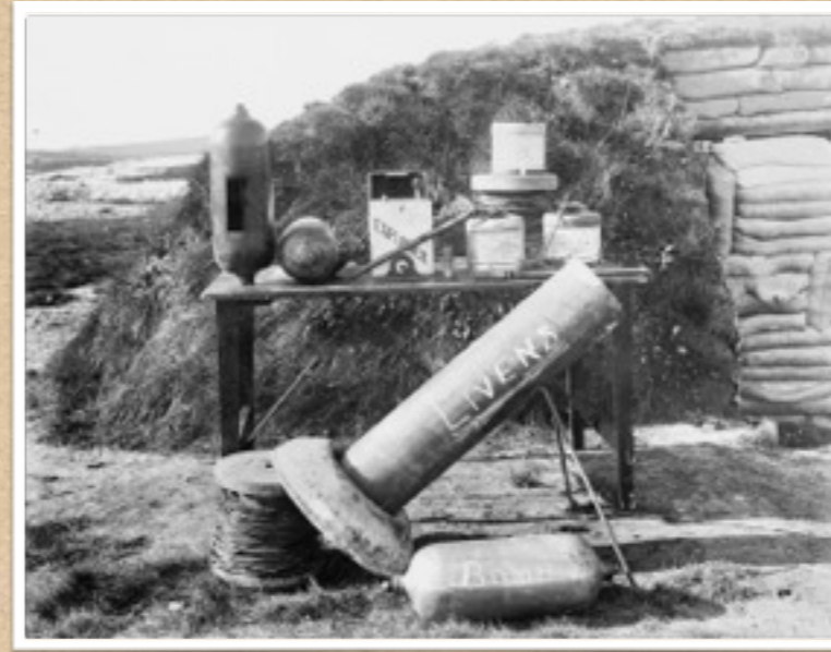
The Livens Projector was a deadly flame thrower that could launch canisters of boiling oil and poison gas into the German trenches. It was devised by a British Army officer from Lincoln . IWM (Q 14940)
