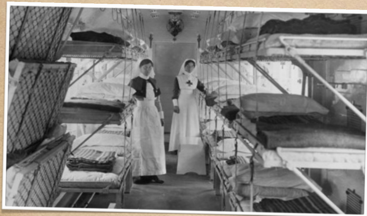
This ingenious three-tier cot system was able to accommodate both seated and lying patients at the same time. It was the brainchild of Frank Marillier, who worked for the Great Western Railway in Swindon in Wiltshire . Photo Courtesy STEAM - Museum of the GWR
